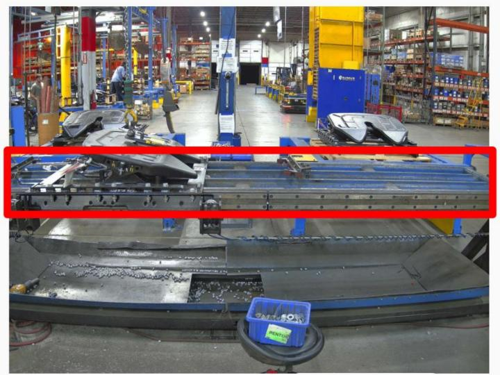
Fifth wheel in assembly, before nuts are tightened.
