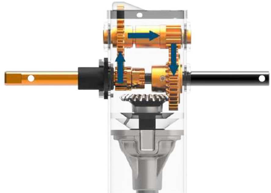
Low Gear 32 Turns / Inch
