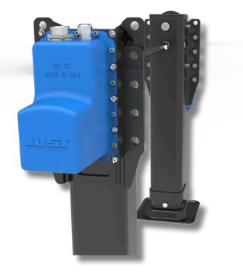
Lifting Capacity: 62,500 lbs<sup>\*\*</sup>
